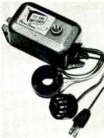
Fig. 10—Perma-Power "Britener" reactivates cathode by raising heater voltage.
